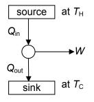
Reasons for the lower efficiencies of practical engines. Maximising use of W and  $Q_{out}$  in combined heat and power schemes.
