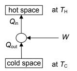
For a refrigerator:  $COP_{ref} = \frac{Q_{out}}{W} = \frac{Q_{out}}{Q_{in} - Q_{out}}$
