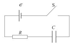
When switch S is closed, the capacitor of capacitance C begins to charge from the cell of emf  $\in$ through the resistor of resistance R. The initial current in the circuit is I.
